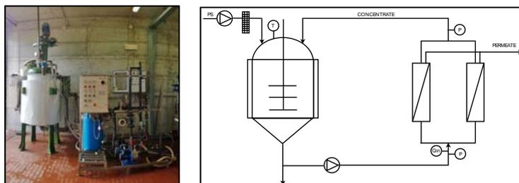
**Fig 1** Integrated pilot scale SAF and membrane separation system
