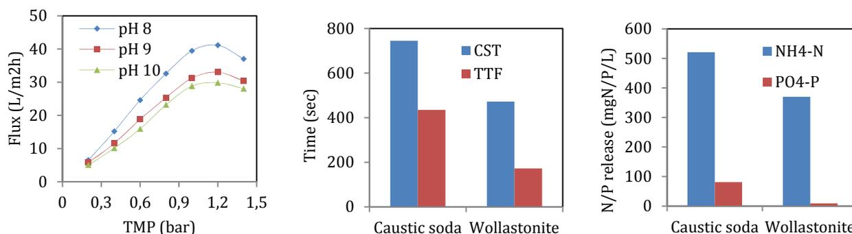
**Fig 3** (a) Effect of pH and TMP on flux (20°C); (b) CST and TTF (dilution 1:5) of SFL for caustic soda (pH 10.0, 40°C) and wollastonite (40 g/L, 37 °C) addition; (c) ammonium and phosphate release for caustic soda (pH 10.0, 40°C) and wollastonite (40 g/L, 37°C)
