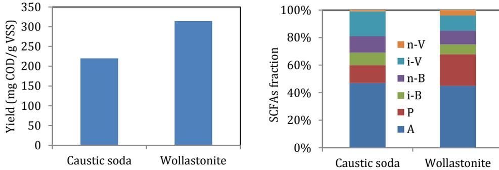
**Fig 2** Comparison between caustic soda (pH 10.0 / 40°C) and wollastonite (40 g/L / 37°C) fermentation experiment: (a) SCFAs production; (b) SCFAs composition.
