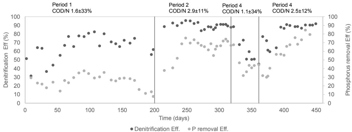
**Figure 6.** Efficiency of denitrification and phosphorus removal during the experimental periods.
