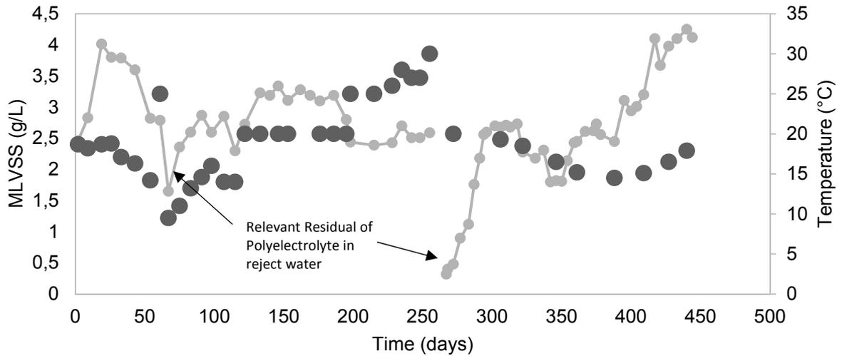
Figure 4. Profile of the environmental temperatures and the MLVSS during the experimental period.
