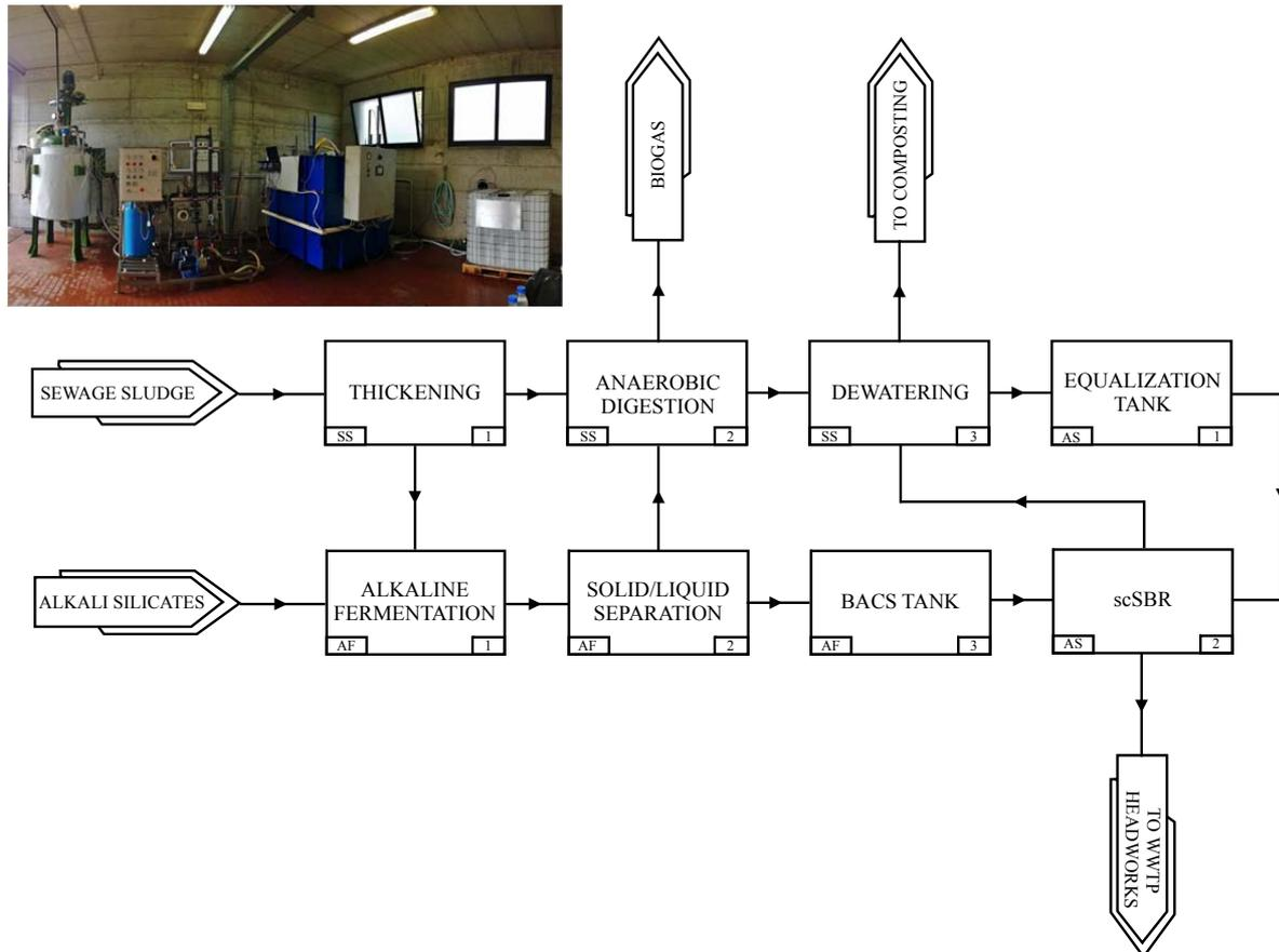
**Figure 1.** Scheme of SCENA system integrated in the Carbonera municipal WWTP. Legend: SS = Sewage Sludge; AF = Alkaline Fermentation; AS = Anaerobic Supernatant. Top left: picture of the pilot-scale SCENA system in the municipal WWTP of Carbonera.
