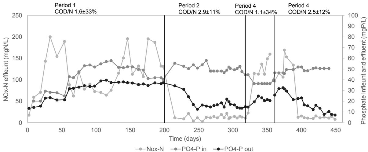
Figure 5. Concentration of the effluent NO<sub>x</sub>-N (mainly nitrite), and the influent and effluent phosphate during the experimental periods
