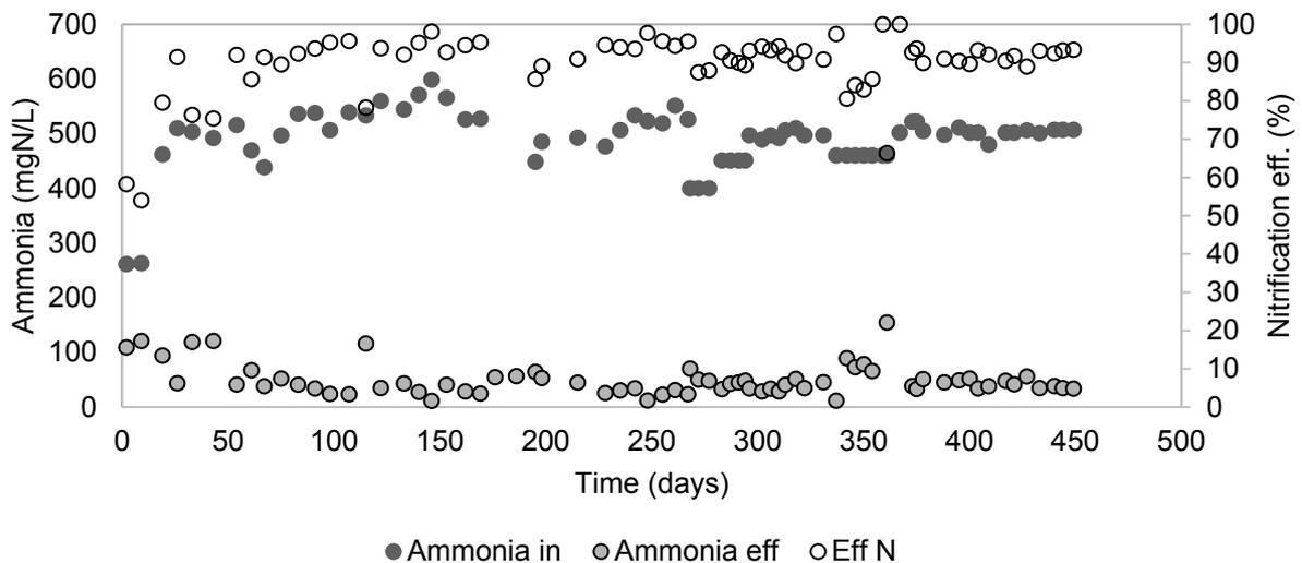
**Figure 3.** Concentration of ammonia influent (anaerobic supernatant), ammonia effluent (treated ammonia supernatant) in the scSBR and nitrification efficiency (Eff% nitrification).
