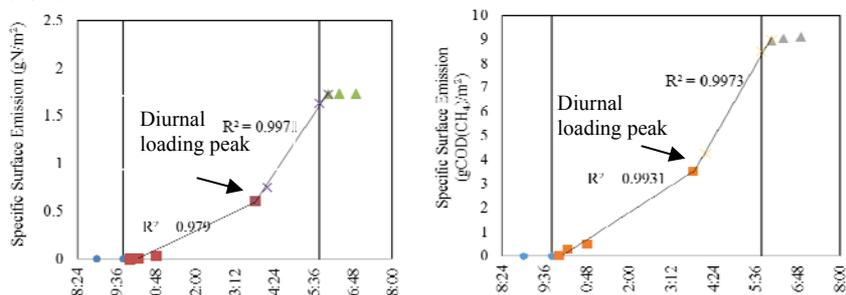
**Figure 2.** Cumulative Specific Surface Emissions of  $N_2O$  and  $CH_4$  during a treatment cycle of intermittent aeration.
