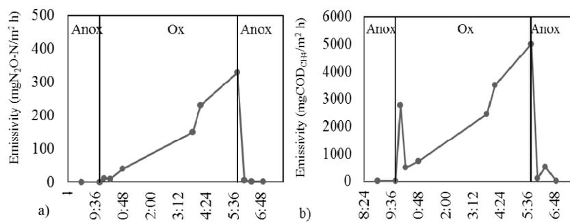
**Figure 1.** Profile of instantaneous emissivity of  $N_2O$  and  $CH_4$  during a treatment cycle of intermittent aeration.
