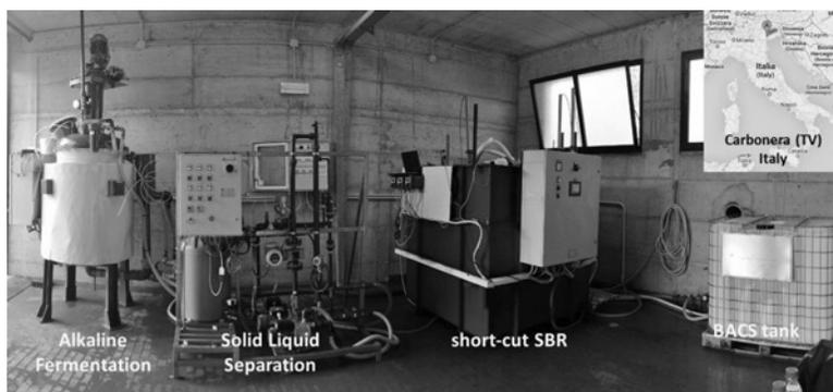
Figure 16.2 Pilot-scale S.C.E.N.A. system.
